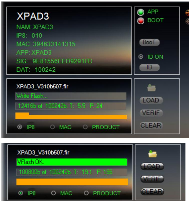
If for any reason during loading a **“Load Flash error”**, not worry, follow these steps: [Load Firmware Error](#) (In the case of SATPRO you may need to increase the parameter `TIMERB = 40`).
