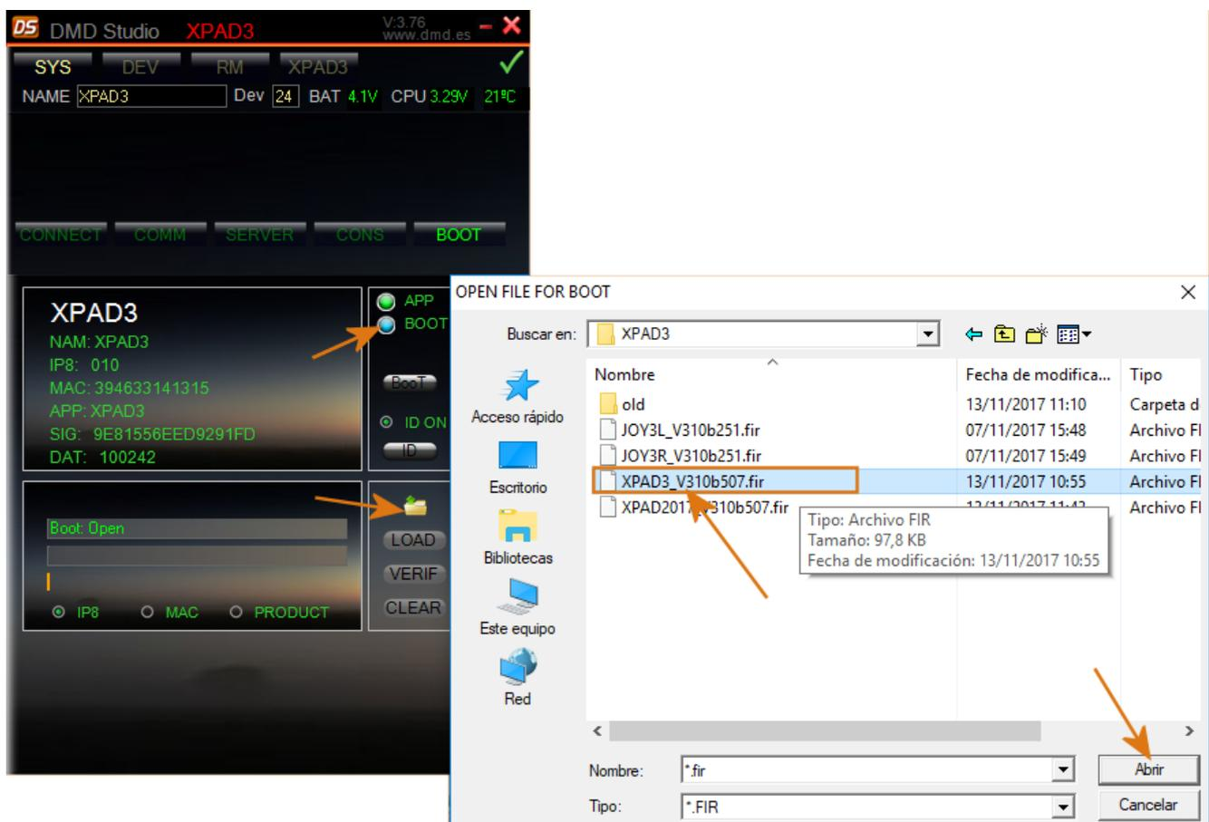
**8- Firmware load.** To load it, we will press the “LOAD” button.
