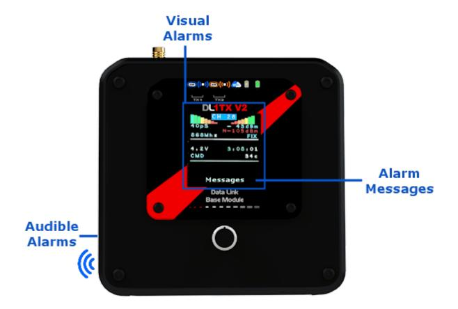
The DL1TXV2 transmitter has several audible alarms, these alarms emit different audible sounds depending on the type of warning.
