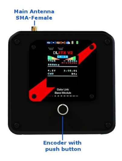
Main Antenna (433Mhz or 863-950Mhz): SMA-Female to connect directional antenna, normally BQ89 biquad antenna, MX433 moxon antenna or omnidirectional antenna. Don't turn on the DL1TXV2 without connecting the antenna.
