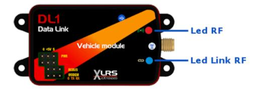
**RF:** RF TX or Packet Transmission, if not linked it sends a data packet every second, once it is linked to an XLRS transmitter the led it will be shown fixed.
