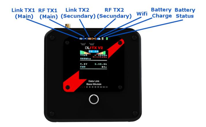
**Link TX1:** It is activated when it has a link with a main receiver XLRS module.
