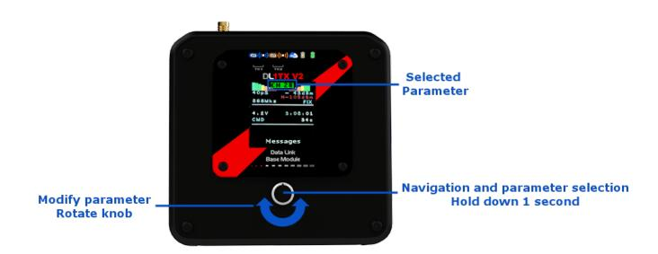
The DL1TXV2 transmitter has a rotary encoder that allows the user to navigate through the different configurable parameters of the device that are shown on the display.
