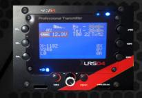
Shows battery status from digital voltmeter or central screen
