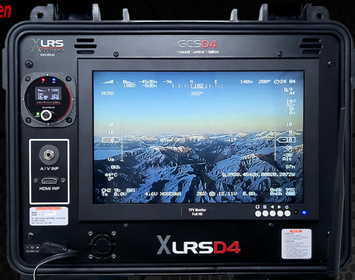
OSD Shows instrumental with Mavlink and XLRs Telemetry
