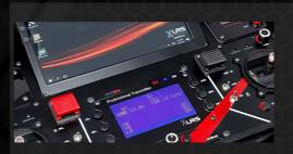
2 Safety Switch with protective cover for some specific safety functions.
