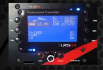
Shows battery status from digital voltmeter or central screen
