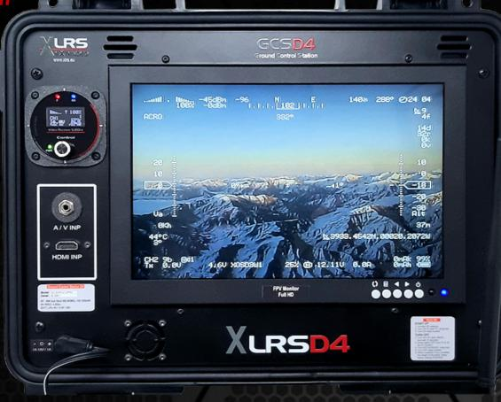
OSD Shows instrumental with Mavlink and XLRS Telemetry
